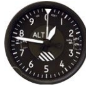
Multi Pointer Long pointer covers 100s Small pointer covers 1000s
