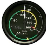
Non-Linear High Range Dial Distance between 20 - 40 kts is more than 120 - 140 kts Also, pointer travels beyond 360°
