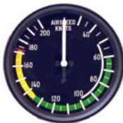
Linear Dial Distance between 20 - 40 kts is same as 120 - 140 kts
